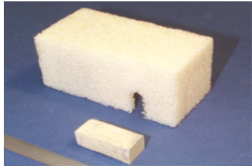
Shape Memory Polymers (SMP) Heat/pressure activation (W. Sokolowski, JPL)
