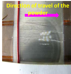
Snapshots from the travel of WCA 12 powder with 50% 7–8.5 \mu\text{m} particles.
